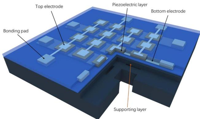
**Figure 2.** 3D schematic of the device.
