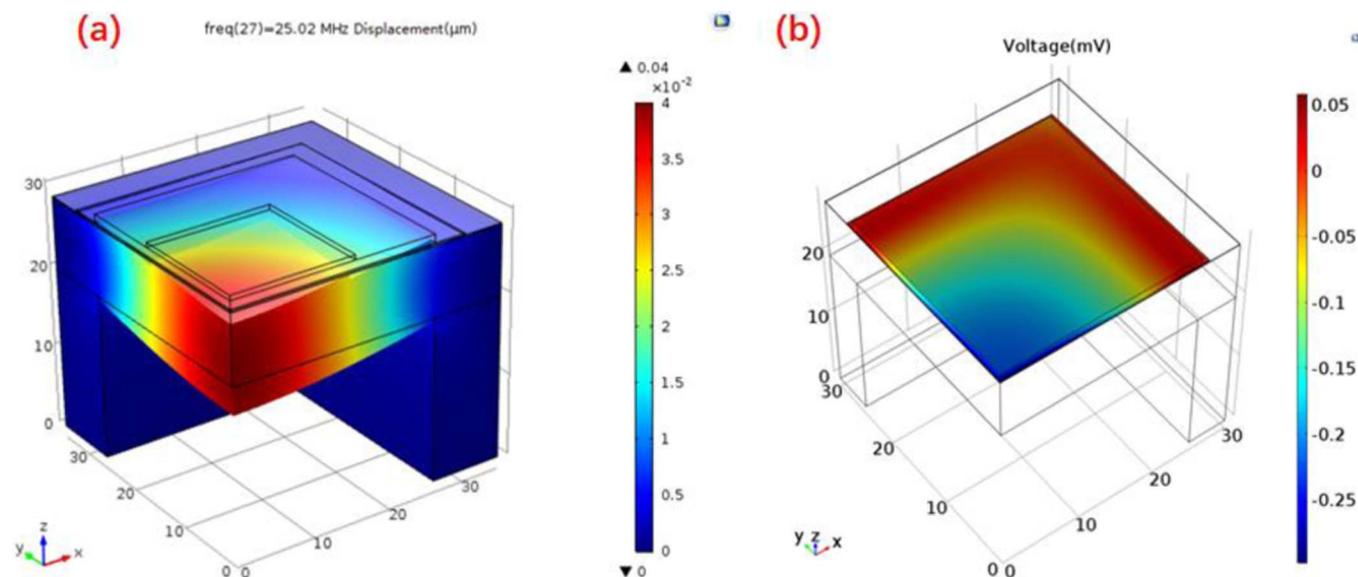
**Figure 3.** (a) The displacement of the membrane at the resonance frequency; (b) The charge density on the membrane in response to an uniform sound pressure.
