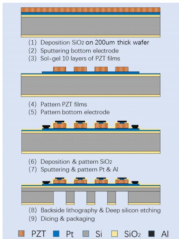
Figure 4. Fabrication process of the device.
