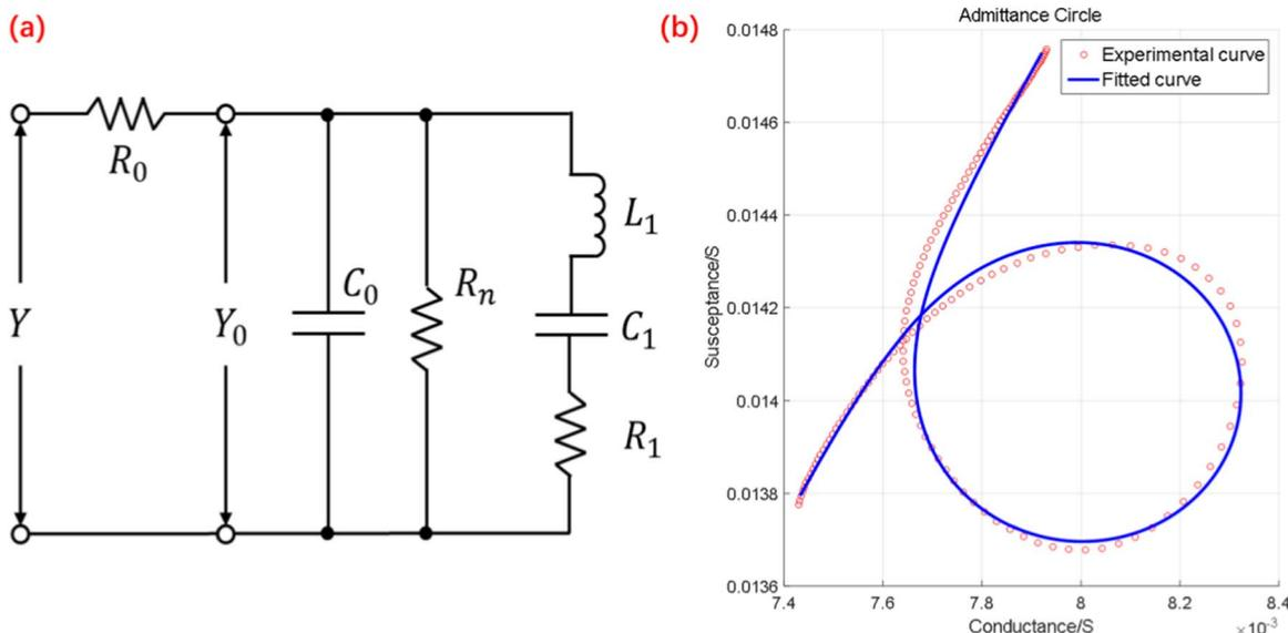
Figure 8. (a) The equivalent circuit of the transducer. (b) The experimental data and fitted result of the admittance circles.
