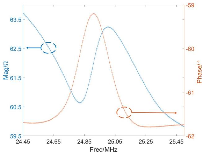
Figure 7. The impedance-frequency spectrum of the pMUT.
