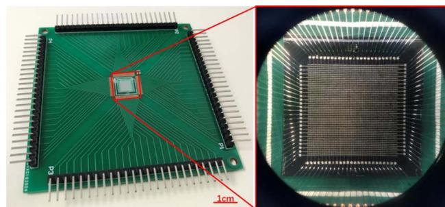
Figure 6. Photo of the packaged pMUTs chip.
