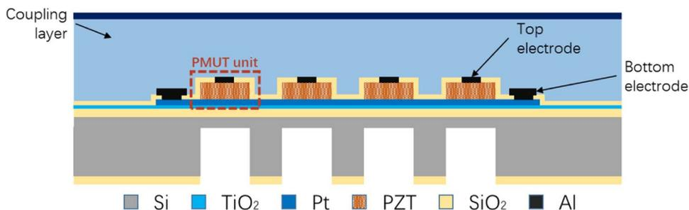
**Figure 1.** Cross-section diagram of the device.
