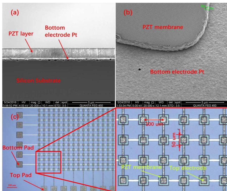
Figure 5. (a) Cross-section SEM image of PZT film. (b) SEM image of isolated PZT membrane with bottom electrode. (c) Optical images of the  $50 \times 50$  pMUT array.
