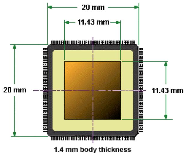
The form factor of the AES4000 is 144-pin JEDEC-standard Low-profile Quad Flat Package (LQFP)
