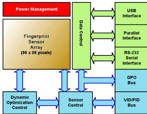
AES4000 EntréPad sensors incorporate flexible *SelectaBus* architecture. This new feature allows the developer to deploy designs that use not only the popular Universal Serial Bus, but also the familiar RS-232 serial interface, or a parallel interface implementation.
