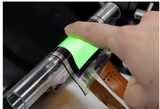
FIGURE 14 Fingerprint image capturing on a flexible display
